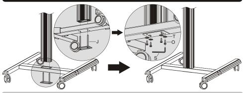
Attach the column to the assembled base using the connecting piece, secure them with the appropriate screws. **NOTE:** Lock the brakes on the casters to avoid any sudden movements during installation.
