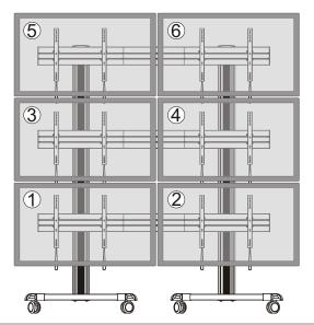
Note: The displays are installed by the numerical order given.
