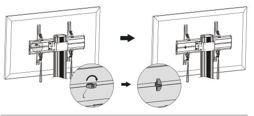
Insert the cable clamps horizontally into the plate slots, then turn the cable clamps to the vertical to secure them.
