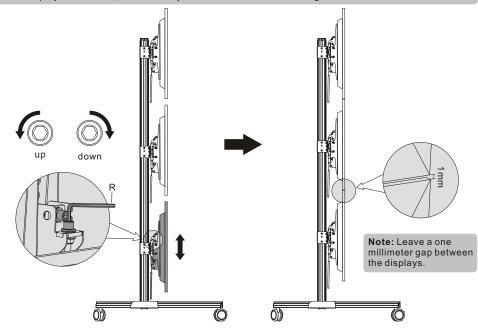
Rotate the adjustment screws as shown in figure to make a one millimeter gap left between the displays.
