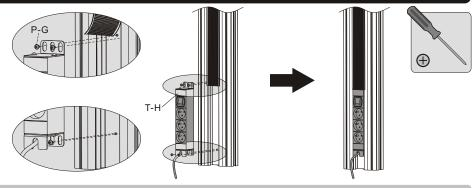
Attach the power socket to the back of column using the appropriate screws. Tighten all screws with a phillips screwdriver.
