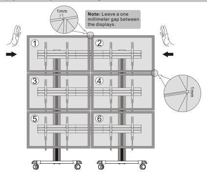
Note: The angle of displays are adjusted by the numerical order given.
